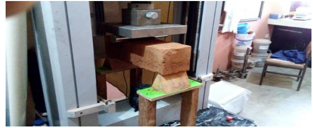
Figure 9. Flexural Test Arrangement
