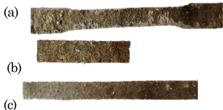
**Figure 1.** Specimen for: (a) tensile testing (b) bending testing (c) impact testing
