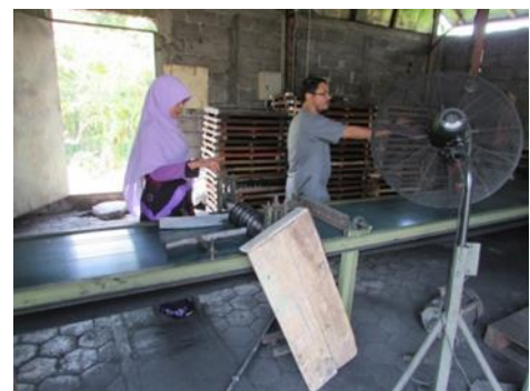
Figure 4 Produced conveyor belt, 8 meters long and 50 cm wide.
