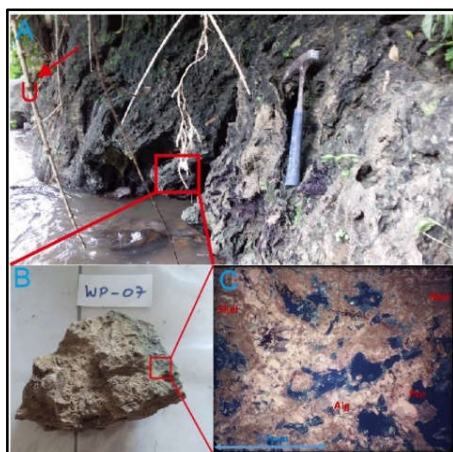
Fig. 5. (A) The outcrop of clastic limestone at STA 32. (B) Handspecimen of clastic limestone, (C) Petrographic appearance of clastic limestone
