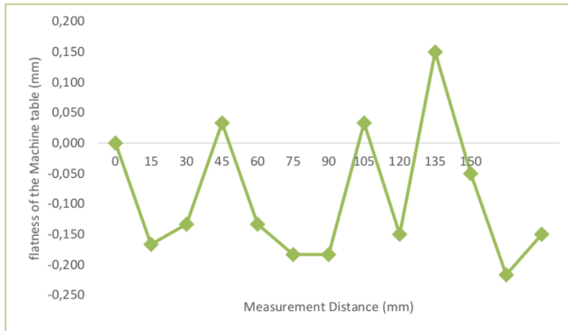
2 Figure 12. Machine table flatness deviation graph.
