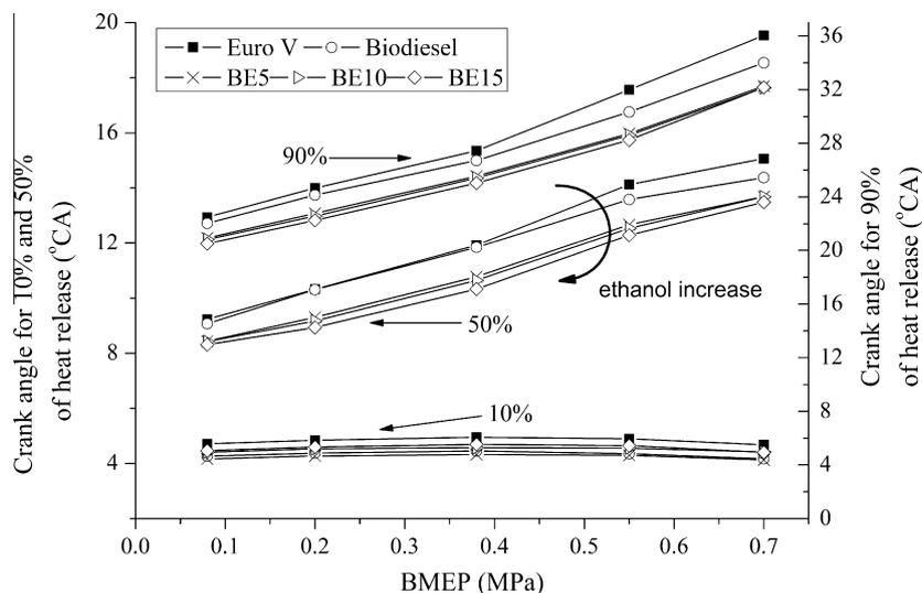
Fig. 4. Crank angle for 10%, 50% and 90% of heat release.
