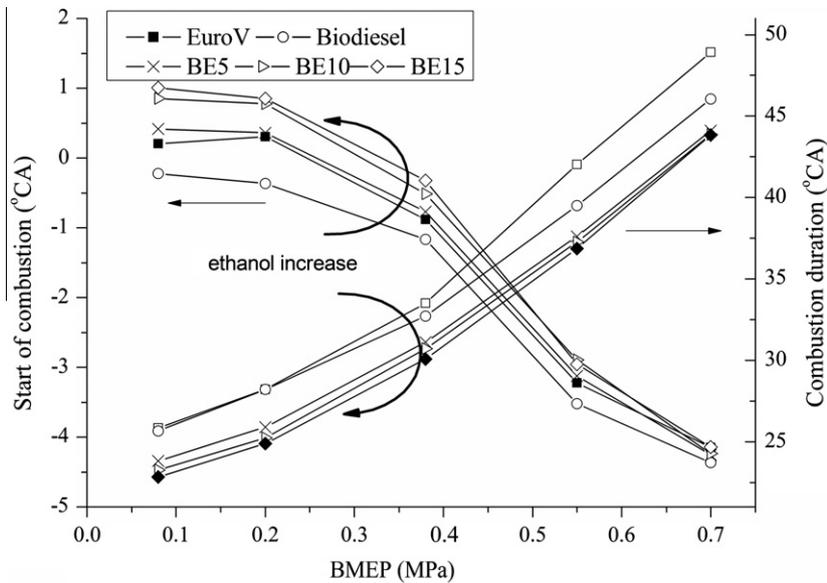
Fig. 3. Start of combustion and combustion duration.
