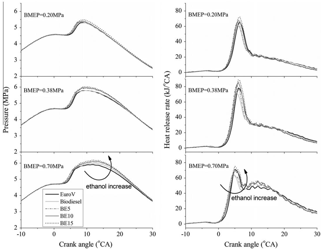
Fig. 2. In-cylinder pressure and heat release rate.
