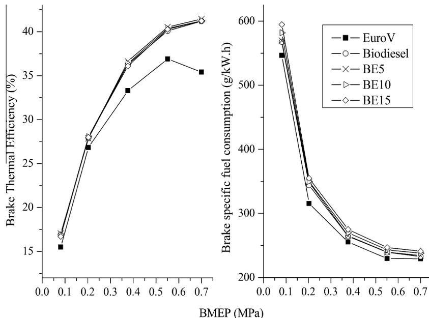
Fig. 5. Brake thermal efficiency and brake specific fuel consumption.
