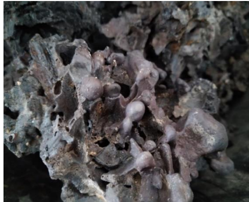
Figure 4. Products with basalt casting with slow cooling
