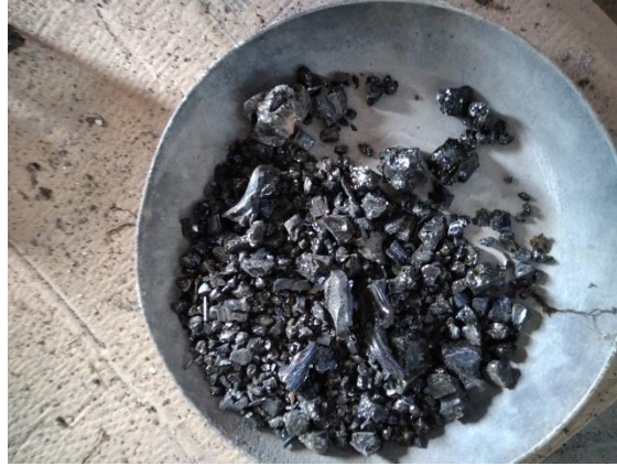
Figure 6. Results of basalt casting products with fast cooling process
