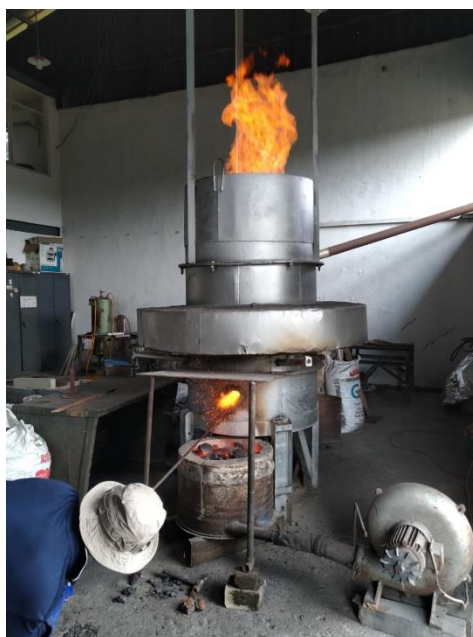
Figure 3. The smelting process of basalt stone in a mini furnace at a temperature of 1500° C
