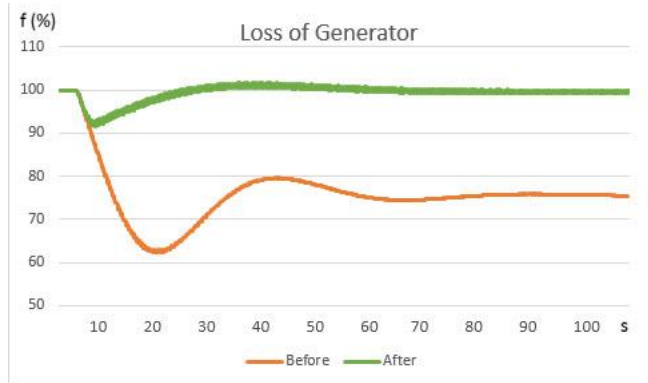
Fig. 6. Frequency response before and after load shedding.
