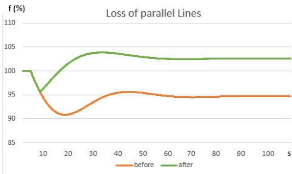
Fig. 4. Frequency response before and after load shedding.
