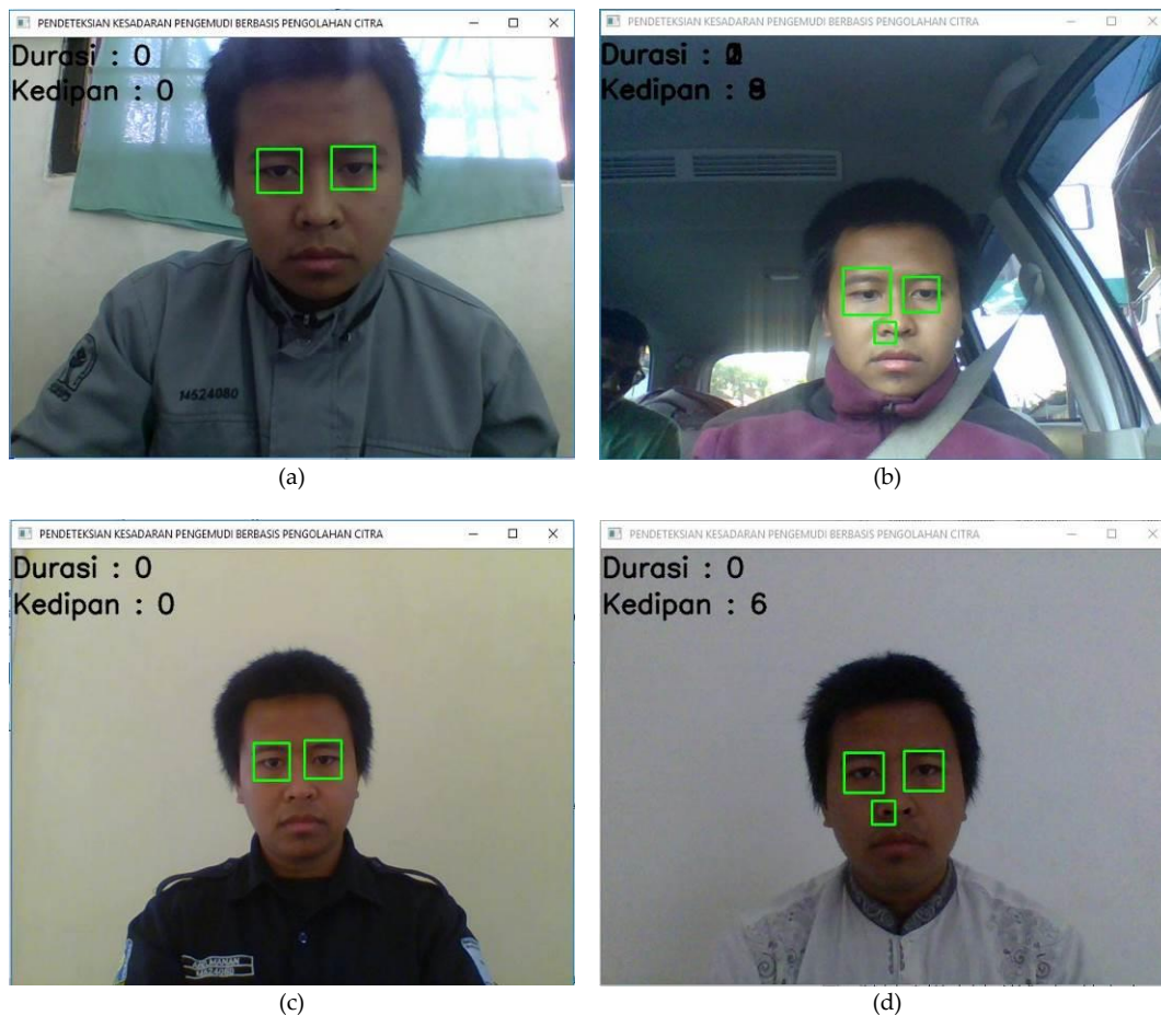
Fig 7. Eye detection based on light
