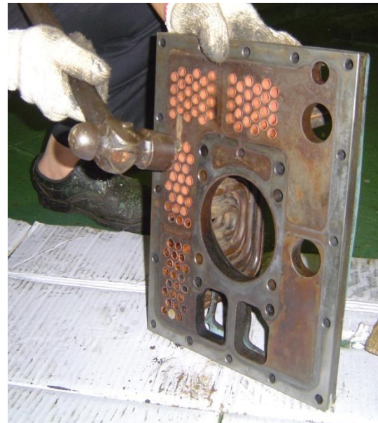
Foto 2. Dinding-dinding pipa intercooler kotor
