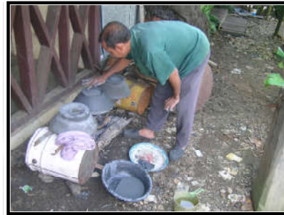
Plate 4. A villager is making large crucibles ( kowi ) for melting brass and other recycled metals (courtesy: Balai Arkeologi Banjarmasin)
