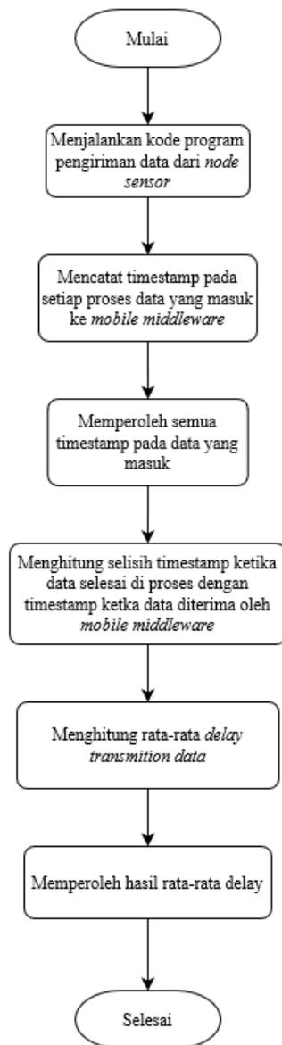
Gambar 3. Diagram Alur Pengukuran Delay Transmission Data
