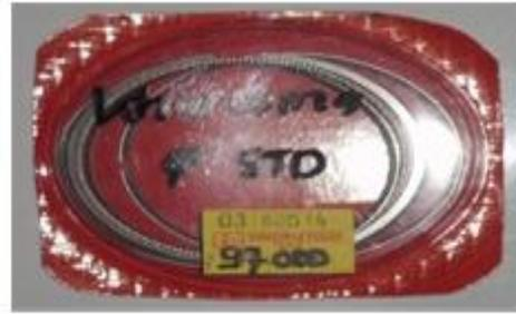
Gambar 4. Ring Piston Original Sepeda Motor Kharisma
