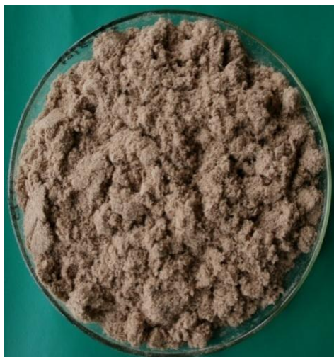
Figure 5. Fiber after organosolv treatment at 170°C and 15 min
