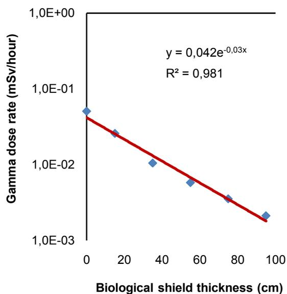
Figure 9. Semi-logarithmic relationship of gamma dose rate against biological shield thickness at HTGR-10 MWth
