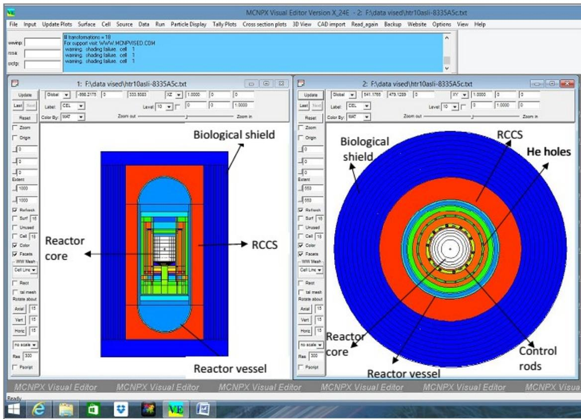
Figure1. Modeling of the HTGR-10 MWth viewed from the side and top of the program package VISED
