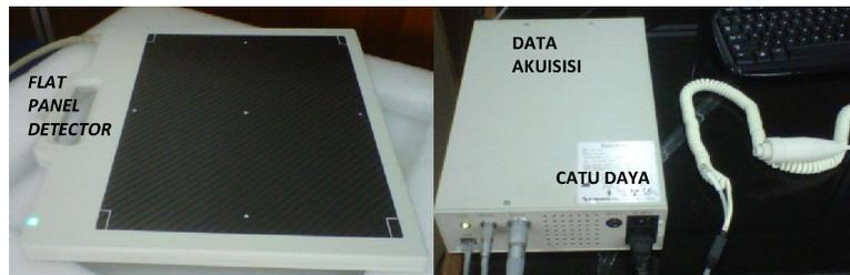
Gambar 3. *Flat-panel detector* DMC-12DR
