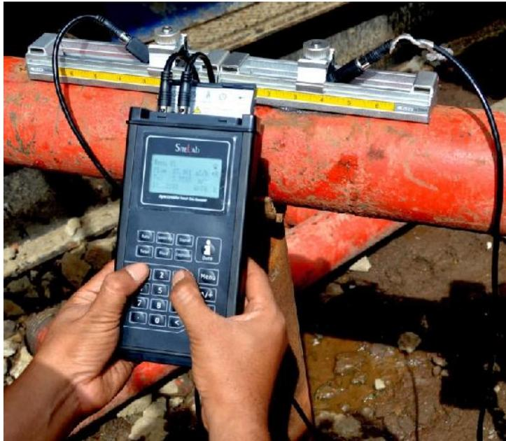
**Gambar 2.1.** *Flow Meter Portable* ([www.flowiratama.com201401flow-meter-air-limbah.html](http://www.flowiratama.com201401flow-meter-air-limbah.html))
