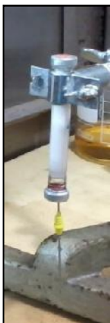
Gambar 2. Kolom ^{188}\text{W}/^{188}\text{Re} berbasis alumina
