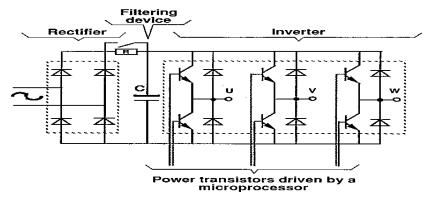
Gambar 3 Blok diagram (Variable Speed Drive) VSD
