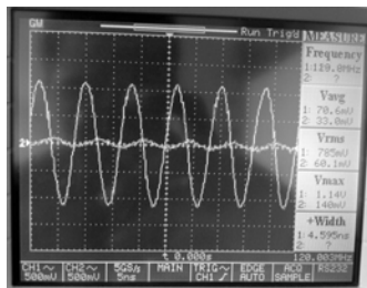
Gambar 4.20 Gambar Gelombang Input dan Output Band Pass Filter
