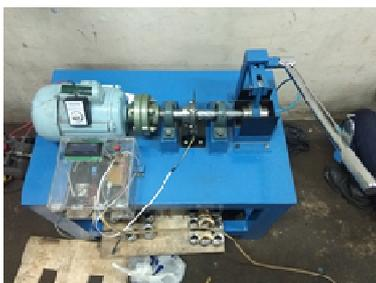
Gambar 3. Prony Brake Dynamometer
