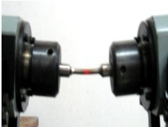
Figure 6. Visual temperature increase for test area of AISI 304 stainless steel at stress 369.53 MPa
