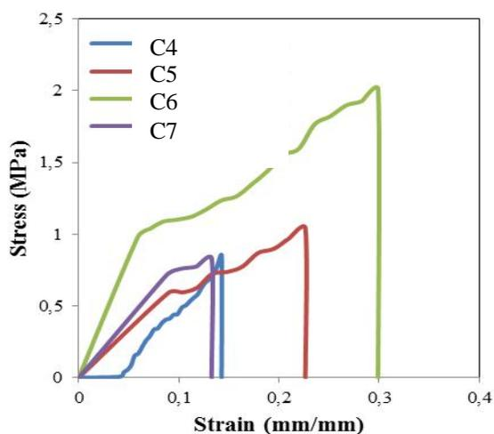
Figure 2. Stress-Strain curve of chitosan-collagen-poly (vinyl alcohol)/bioceramic composites.
