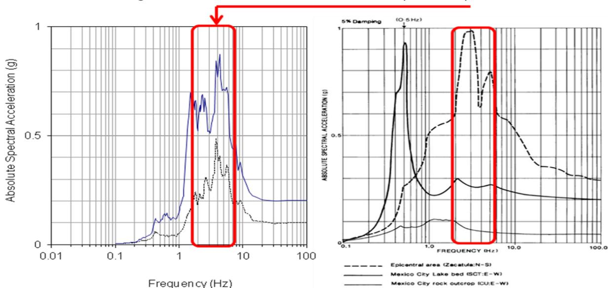
Figure 11. Frequency domain of response spectra at soil level at SMK – Dirmutala Stadium, Banda Aceh
