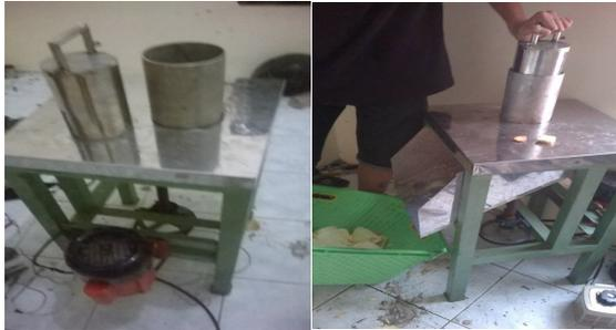
**Gambar 2. Alat Pemotong Ceriping Ubi Jalar**
