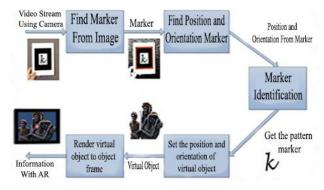
Figure 2: Augmented reality procedure.
