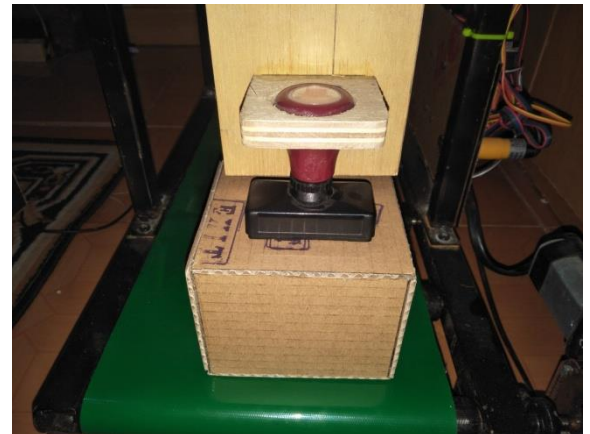
Figure 14 Label Stamping Process
