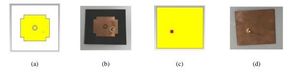
Figure 2. Design of a truncated slotted ring patch antenna, (a) imulation (top view), (b) fabrication (top view), (c) simulation (bottom view), (d) fabrication (bottom view) [16]
