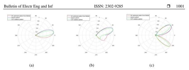
Figure 11. Beam steering technique of the radiation pattern of 1×4 truncated-slotted ring antenna array using AEP and GA towards (a) 10°, (b) 20° and (c) 30° [16]
