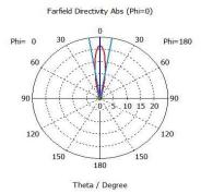
Figure 10. Radiation pattern of 1 by 4 truncated-slotted ring antenna array [16]
