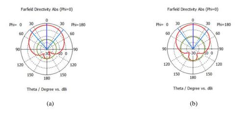
Figure 8. Radiation pattern of a (a) slotted ring, (b) truncated slotted ring patch antenna[16]
