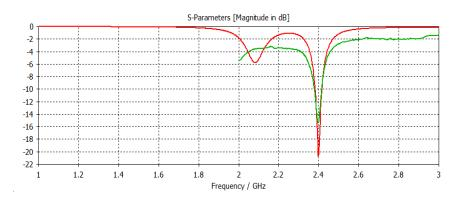
Figure 7. Simulated S<sub>11</sub> (red curve) and measured S<sub>11</sub> (green curve) of a truncated slotted ring patch antenna [16]
