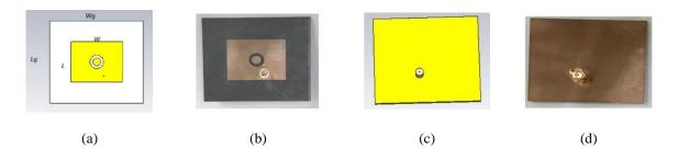
Figure 1. Design of a slotted ring patch antenna, (a) simulation (top view), (b) fabrication (top view), (c) simulation (bottom view), (d) fabrication (bottom view)
