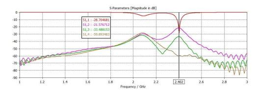
Figure 9. S-parameters of a truncated slotted ring patch antenna [16]
