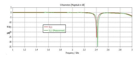
Figure 6. Simulated  $S_{11}$  (red curve) and measured  $S_{11}$  (green curve) of a slotted ring patch antenna
