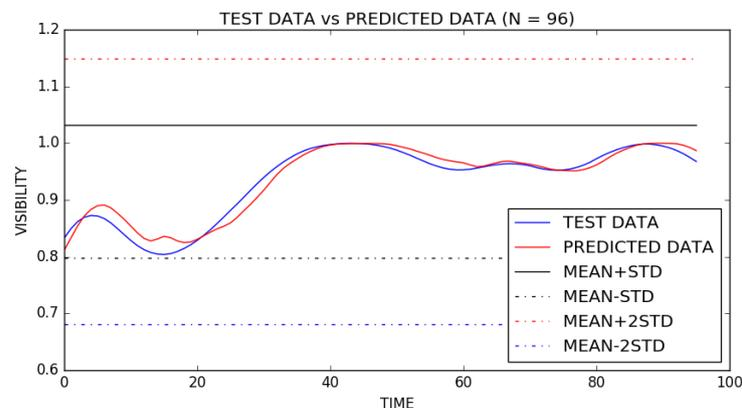
Figure 7. Comparison between predicted visibility for 96 future points and actual test visibility dataset using the trained merged-LSTM
