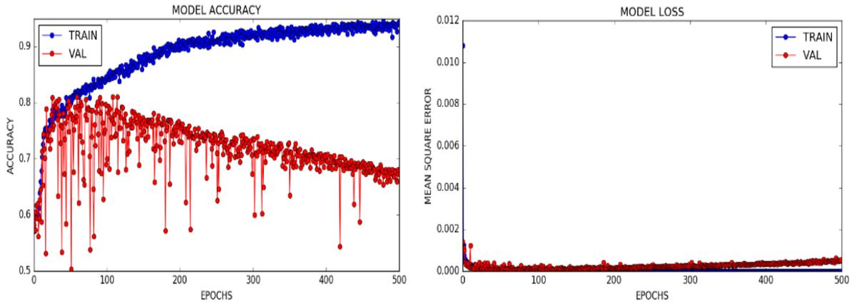
Figure 5. Training accuracy and loss of model merged-LSTM with temperature and dew point as moderating variable
