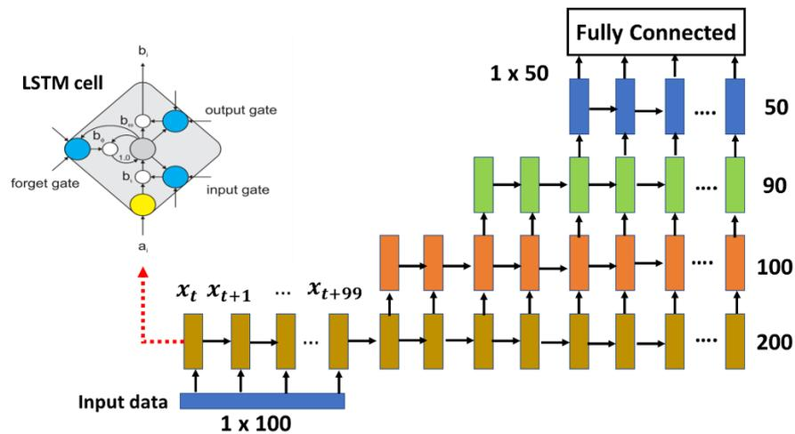
Figure 2. Structure of LSTM model
