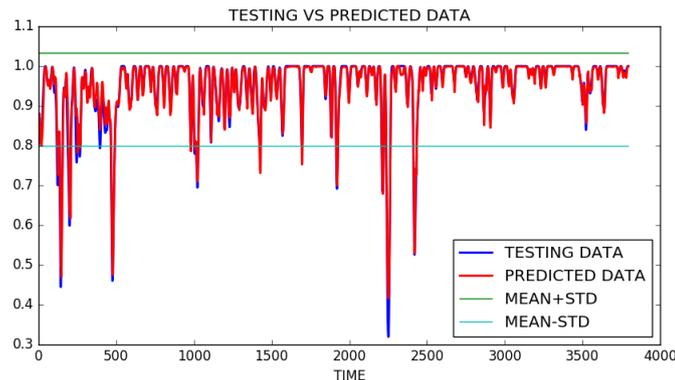
Figure 6. Comparison between predicted visibility and actual test visibility dataset using trained merged-LSTM
