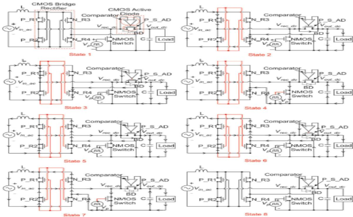
Figure 2. Switching algorithm in proposed CMOS rectifier with boost converter [11]
