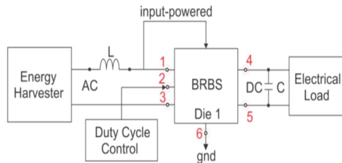
Figure 1. Block diagram of CMOS rectifier with Boost-Converter (BRBS) presents the input-powered converter, which eliminated the pre-charged of the load [11]
