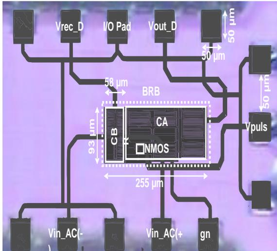
Figure 6. Photomicrograph of the fabricated rectifier (BRBS) in 0.18 μm CMOS technology
