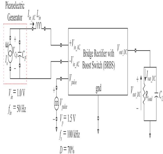
Figure 7. Measurement setup
