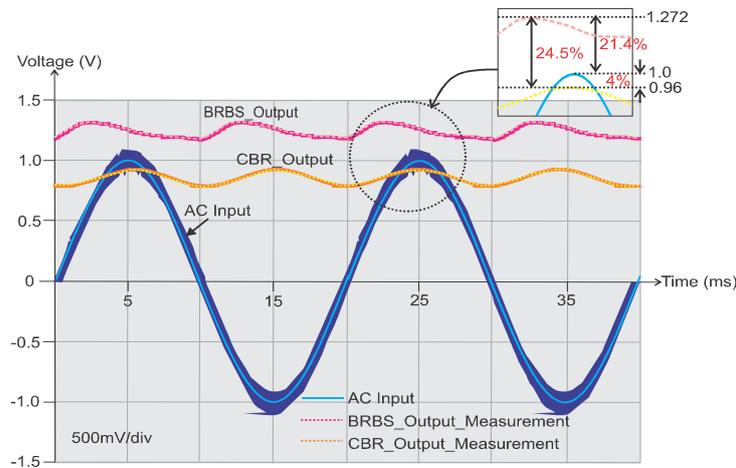
Figure 8. Measured output voltages of the proposed CMOS Rectifier without Boost-Converter (CBR) and CMOS Rectifier with Boost-Converter (BRBS) circuits
