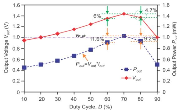
Figure 5. Simulated output voltage and output power with variation of duty cycle
