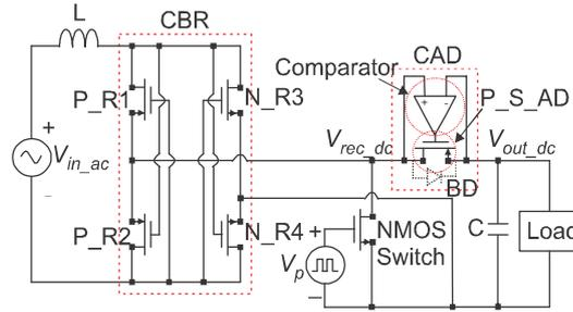
Figure 3. NMOS and PMOS are used as the switching devices in the proposed CMOS Rectifier with Boost-Converter (BRBS) based on 0.18 μm CMOS process technology
