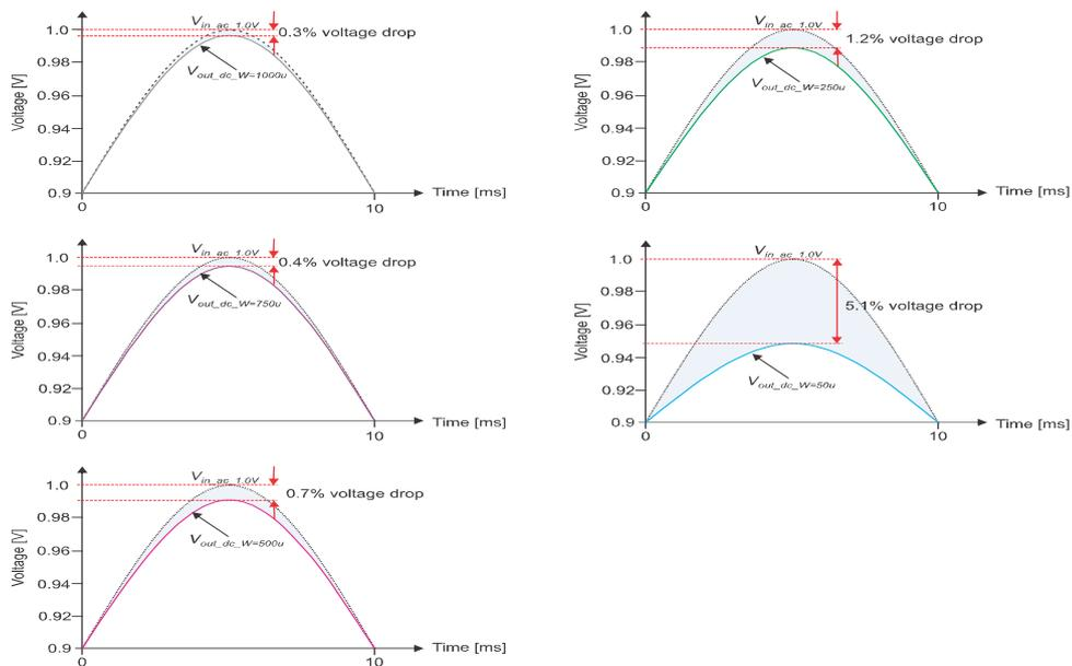
Figure 4. Simulated output voltage with the voltage drop for different size of MOSFETs in the proposed rectifier.  $V_{in}=1.0$  Vac,  $f_{in}=50$  Hz and  $R_{load}=2$  k $\Omega$
