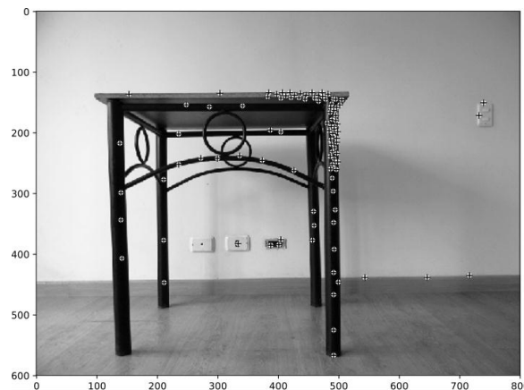
Figure 3. Image of the left camera converted to grayscale, scaled to 800 \times 600 and with the bacteria overlapped in its final position, most of them on the obstacle
