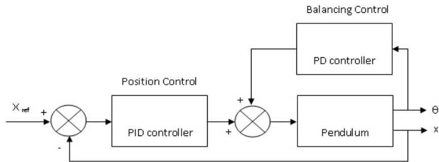
Figure 6. PID controller based pendulum balancing of linear servo system
