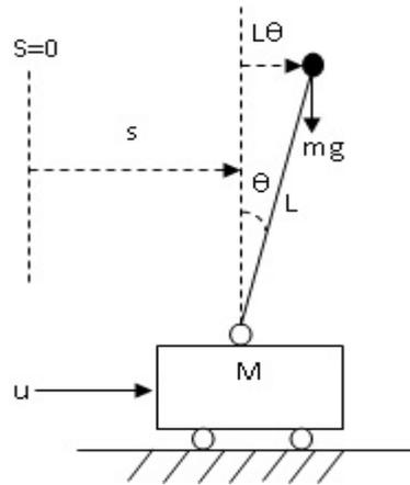
Figure 1. Inverted pendulum on a carriage
