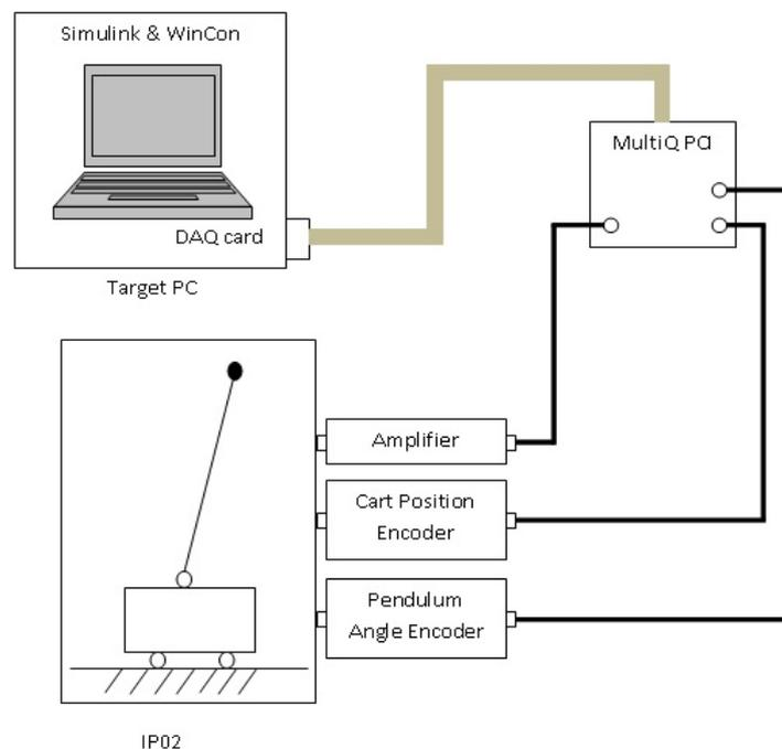
Figure 5. Serial connection between host and target computer to the pendulum system (IP02)
