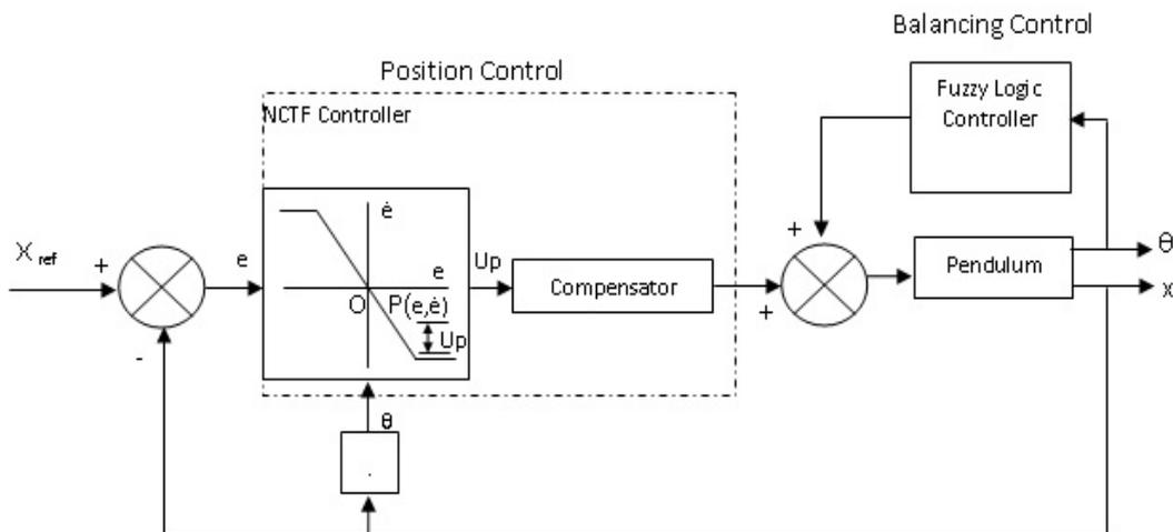
Figure 7. Proposed practical controller structure
