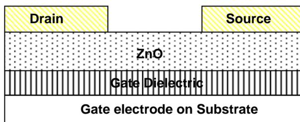
Figure 2. Bottom gate ZnO thin film transistor
