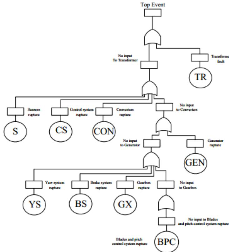
Figure 4. Fault tree for the wind turbine
