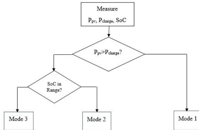
Figure 4. Flow chart of charging mode of operation
