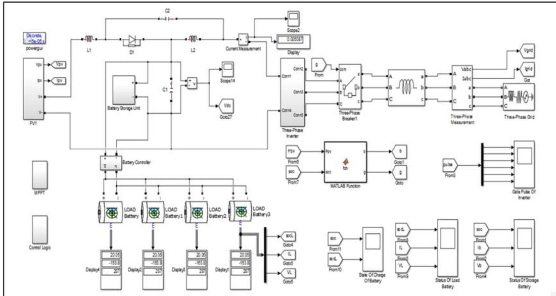
Figure 3. Overall MATLAB circuit diagram for bidirectional vehicle charging station using qZSI PV inverter
