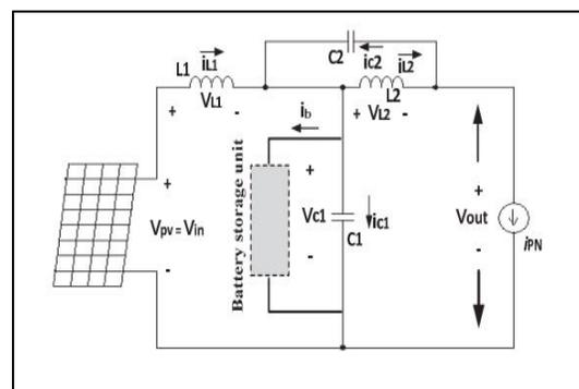
Figure 2. Equivalent circuit of non-shoot through state
