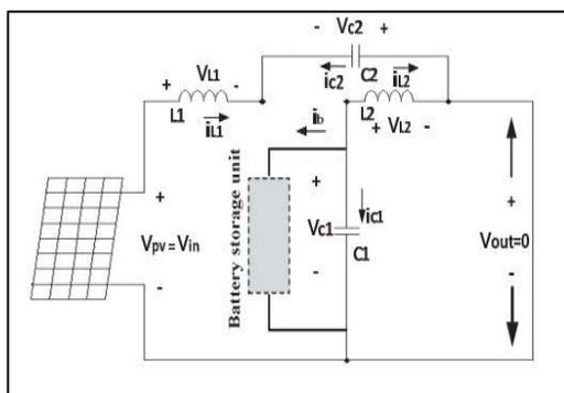
Figure 1. Equivalent circuit of shoot through state
