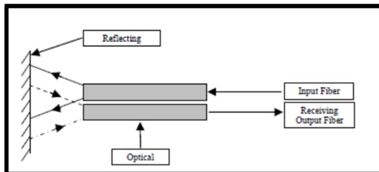
Fig. 3. Two fibers displacement sensor technique
