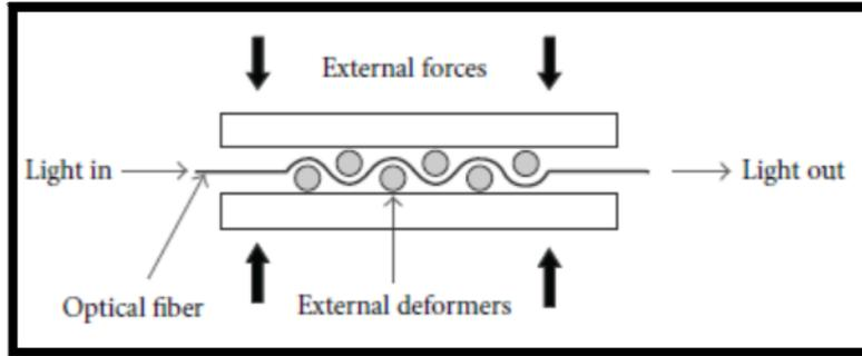
Fig. 4. Microbends sensor structure [6]
