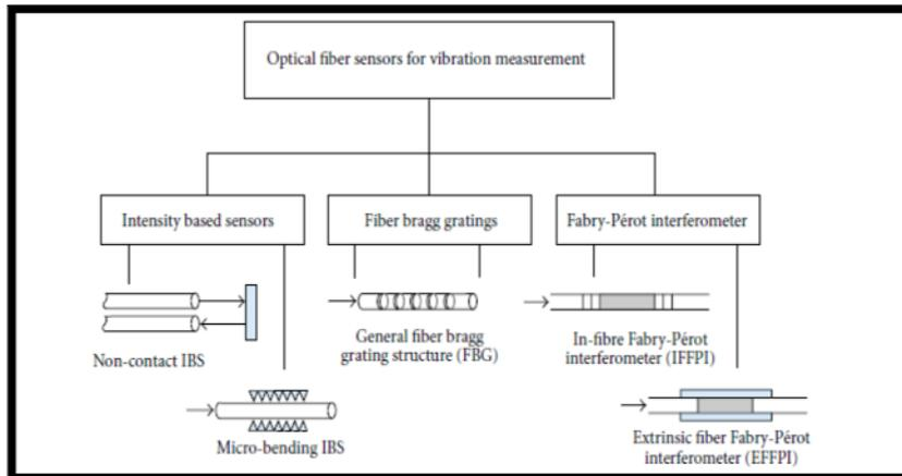
Fig. 2. Vibration optical fiber sensors classification [2]
