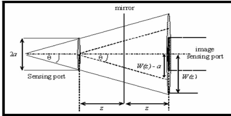
Fig. 6. Evaluating scheme for power light emitted and received by fiber
