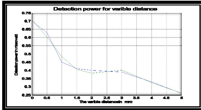
Fig. 11. Plotting power light received by detector with respect to mirror's displacement
