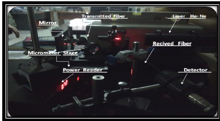
Fig. 8. shows the photograph of experimental setup
