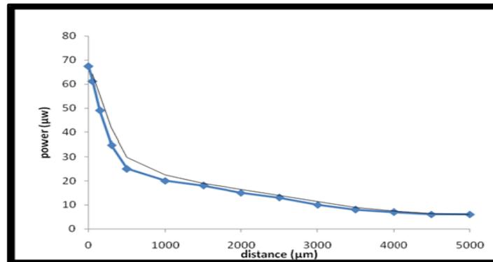
Fig. 12. Theoretical result between variable distance against output power
