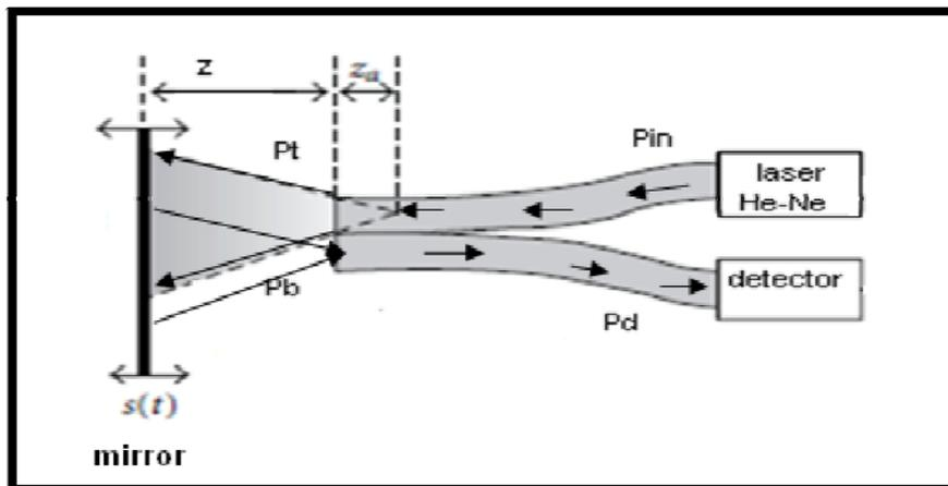
Fig. 5. The basic setup for displacement sensor using multimode fiber
