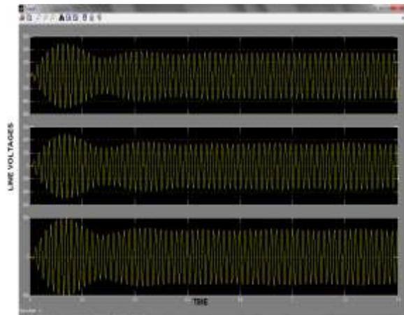
Figure 7. Output waveform of Quasi Z source Inverter for SPWM Technique
