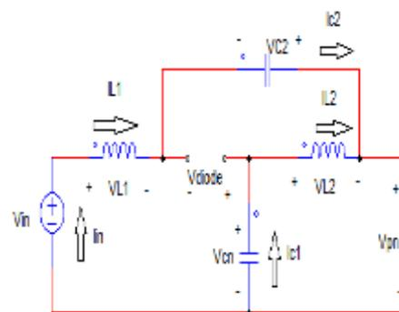
Figure 2. Shoot through Equivalent Circuit
