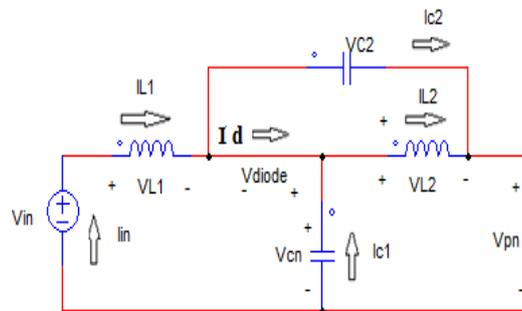
Figure 3. Non-Shoot through Equivalent Circuit
