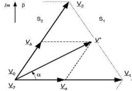
Figure 6. Space Vector Modulation principle
