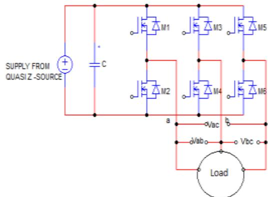
Figure 4. Three Phase Inverter
