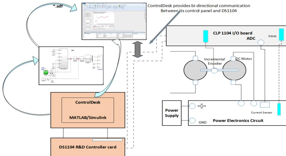
Figure 3. Setup for wind turbine emulator
