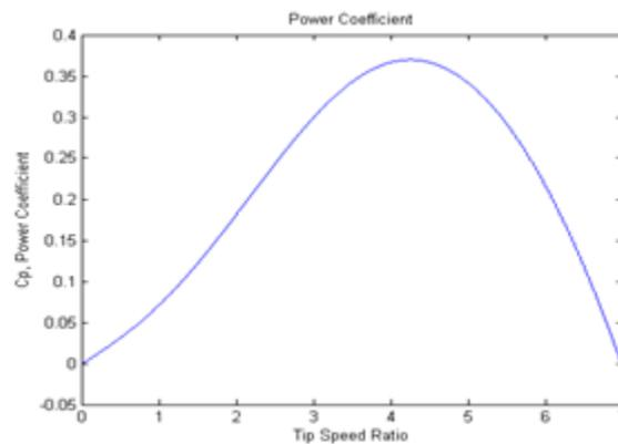
Figure 1. Power co-efficient ( $C_p$ ) vs Tip Speed Ratio ( $\lambda$ )
