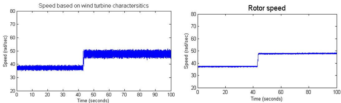
Figure 2. The performance of the developed WTE, (a) speed based on turbine characteristics (b) motor speed (rad/sec)
