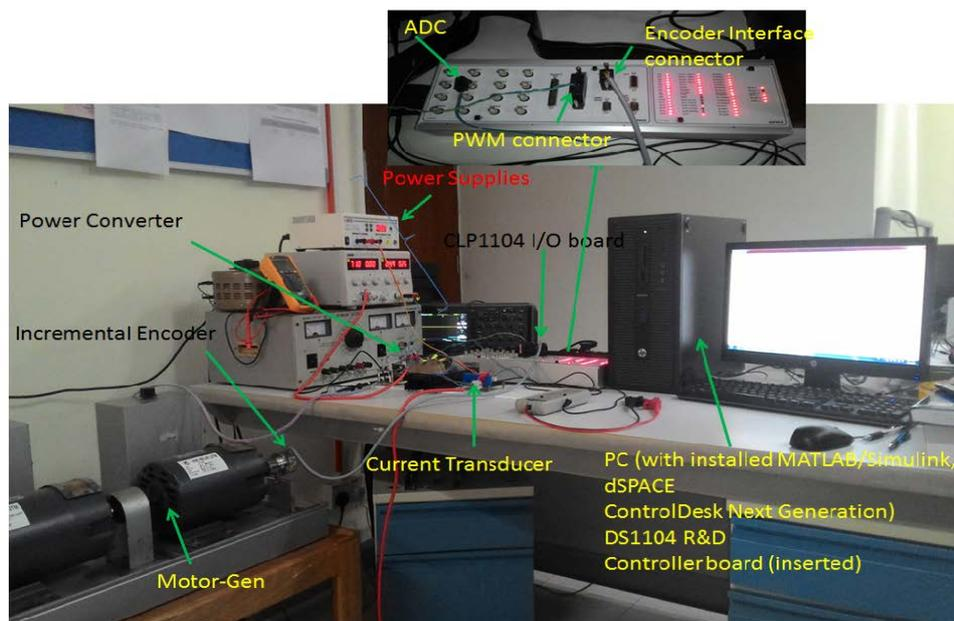
Figure 2. Developed wind turbine emulator
