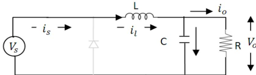
Figure 2. Equivalent Circuit during ON State
