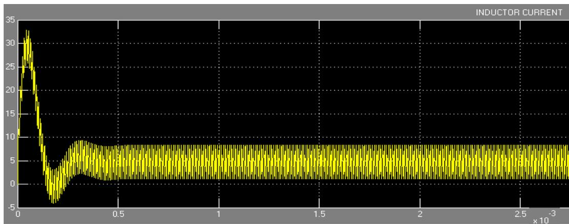
Figure 12. Inductor Current waveform of buck converter using Open Loop model
