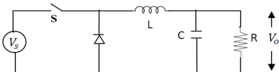
Figure 1. Circuit Diagram of Buck Converter
