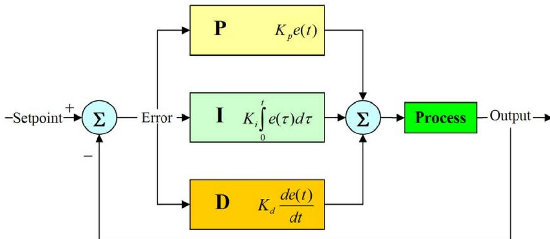
Figure 5. Block Diagram of a PID Controller
