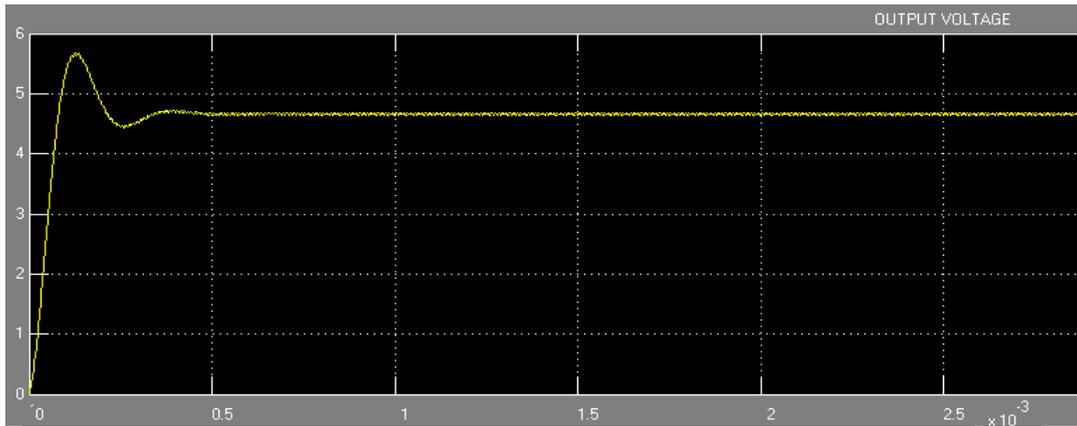
Figure 11. Output Voltage waveform of buck converter using Open loop model
