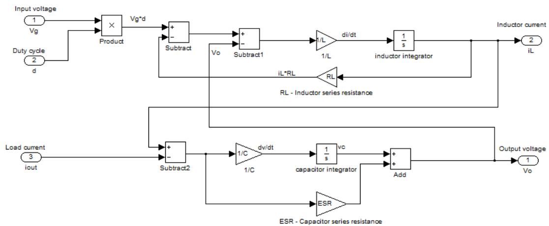
Figure 10. Subsystem of Buck Converter
