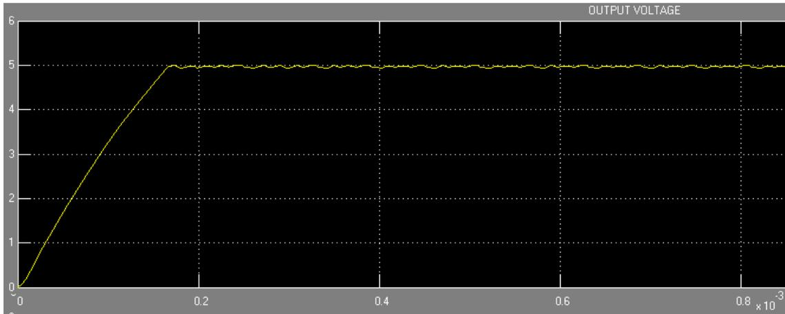
Figure 14. Output Voltage waveform of buck converter using PI Controller
