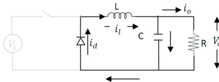
Figure 3. Equivalent Circuit during OFF State
