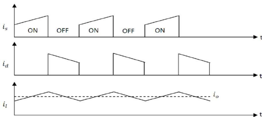
Figure 4. Waveforms of Buck Converter
