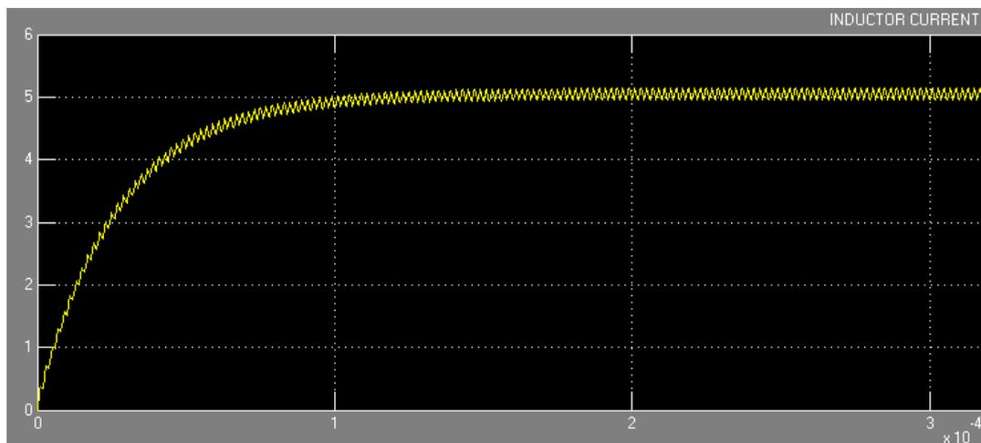
Figure 18. Waveform of Inductor Current of Buck Converter using Fuzzy Controller
