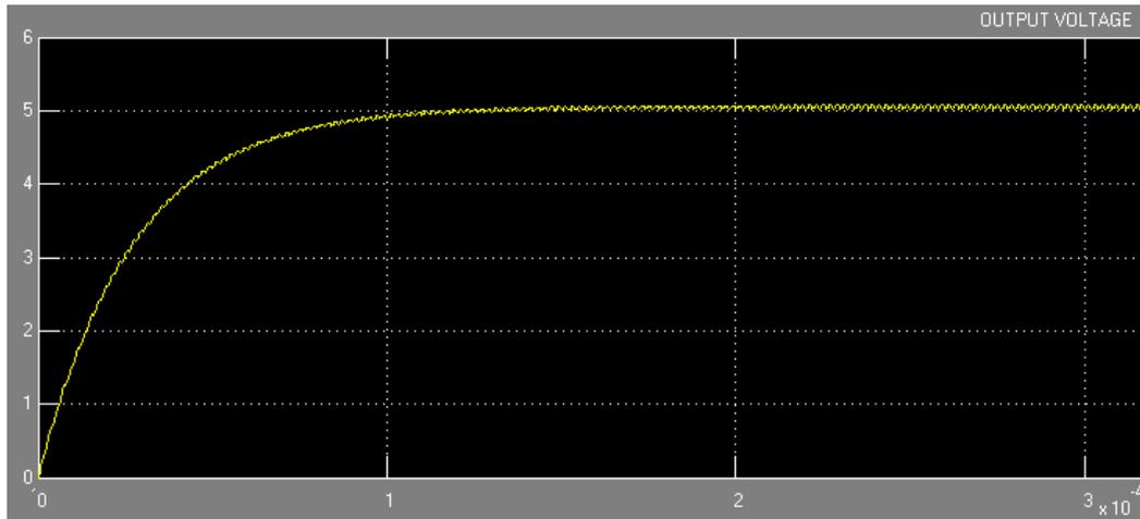
Figure 17. Waveform of Output Voltage of Buck Converter using Fuzzy Controller
