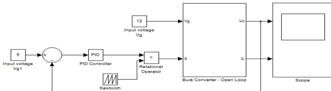
Figure 13. Closed loop model of Buck Converter using PI Controller.
