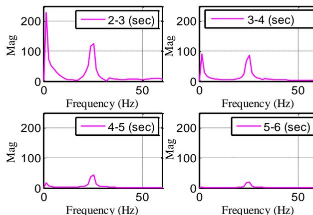
Figure 10. FFT analysis on rotor speed deviations when proposed compensator is enhanced with auxiliary damping controller
