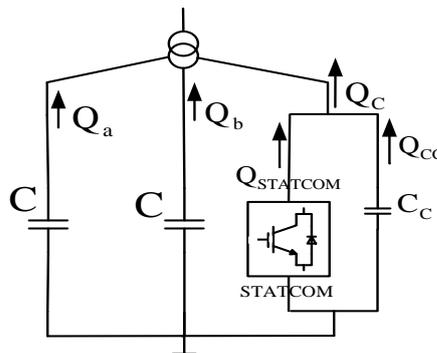
Figure 2. Schematic diagrams of the hybrid shunt compensation schemes
