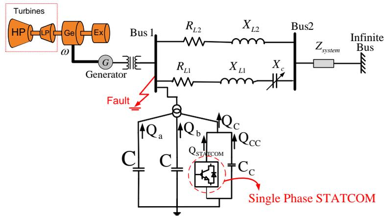
Figure 3. The IEEE second benchmark model combined with unbalanced shunt compensator for SSR analysis
