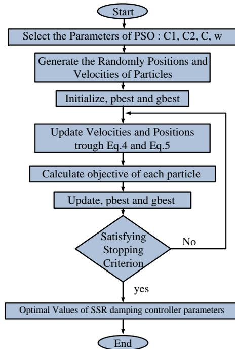
Figure 8. Flowchart of the PSO algorithm
