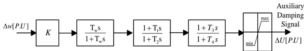
Figure 7. SSR damping controller block diagram
