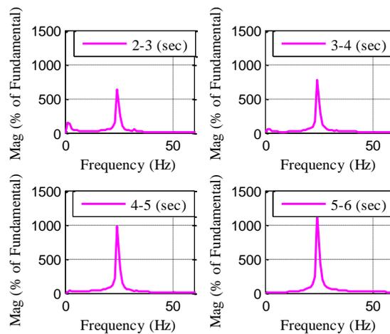
Figure 5. The FFT analysis on the generator rotor speed without damping controller in 2-6 sec with the time division of 1 second
