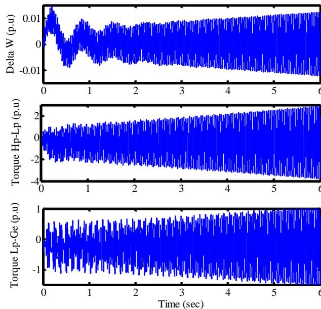
Figure 6. Simulation results for the IEEE-SBM without controllers
