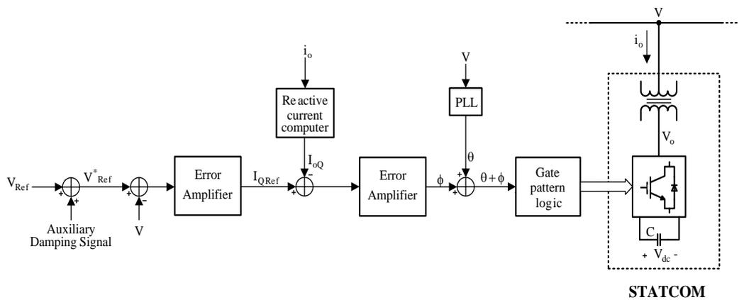
Figure 1. STATCOM control system
