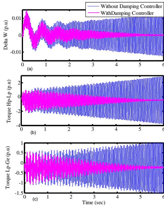
Figure 9. Simulation results for SSR damping with proposed unbalanced shunt compensator. (a) The generator rotor speed deviation (b) The torques between high pressure and low pressure turbine and (c) The torques between generator and low pressure turbine with and without damping controller
