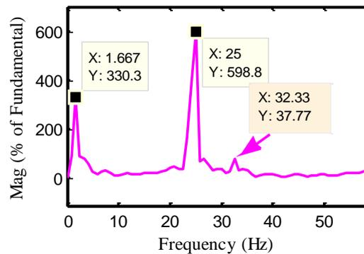
Figure 4. FFT analysis on generator rotor shaft in order to confirm the dominant mode
