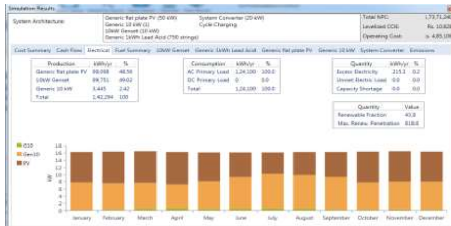
Figure 12. Monthly average electrical energy production from different elements of hybrid system
