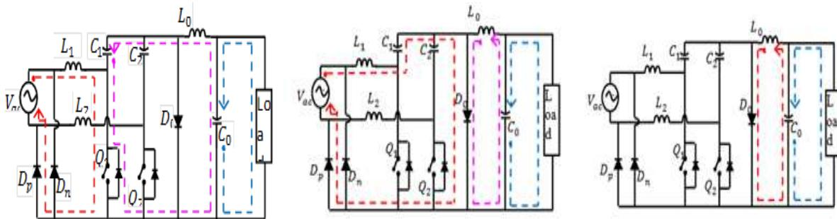
Figure 3(a). Mode 0 operation during positive half-cycles of the supply voltage
