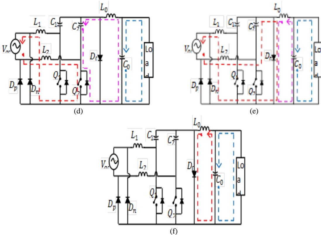
Figure 3(d)-(f). Modes of operation during negative half-cycles of the supply voltage
