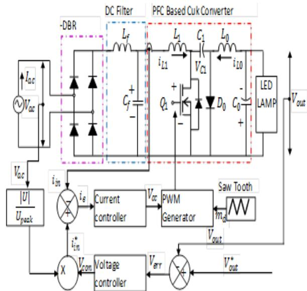
Figure 1. The traditional PFC Cuk converter-based LED lamp driver
