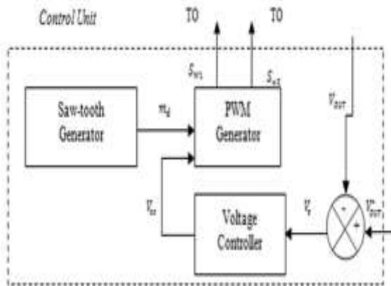
Figure 5. Control unit (Voltage Follower Approach) of MBL-CUK CONVERTER
