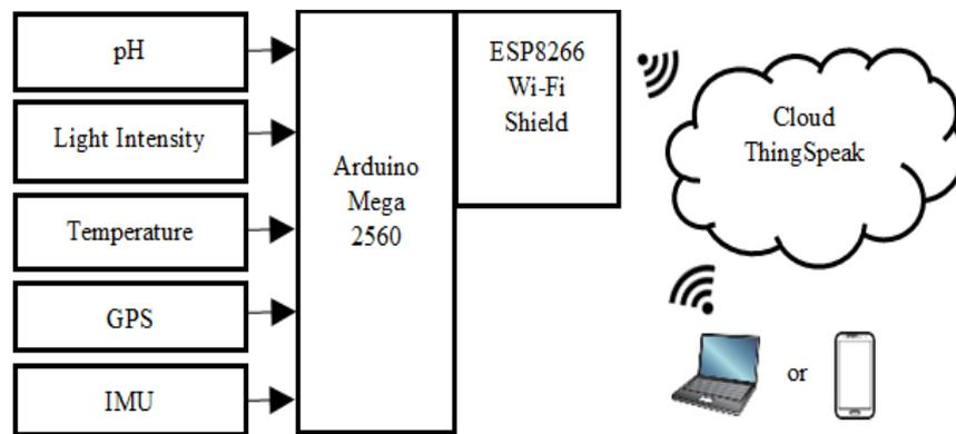
Figure 1. Block diagram
