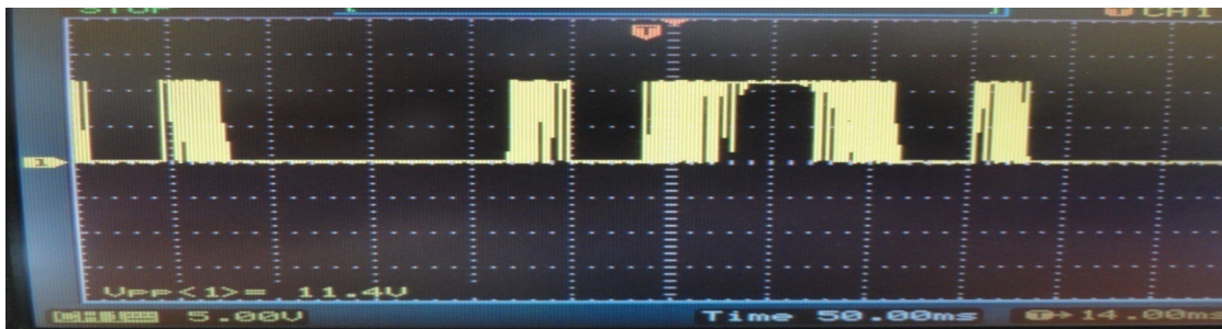
c. Gating pattern for the switch S_3 (the switching pattern obtained from portB of PIC18F4550)
