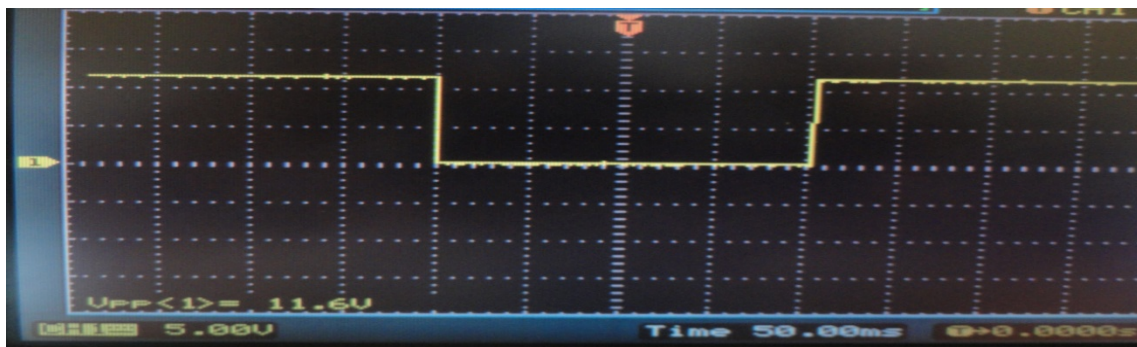
e. Gating pattern for the switch S_5 (the switching pattern obtained from portB of PIC18F4550)
