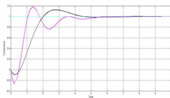
Figure 8. Comparison of ZN and MZN tuned PI controller
