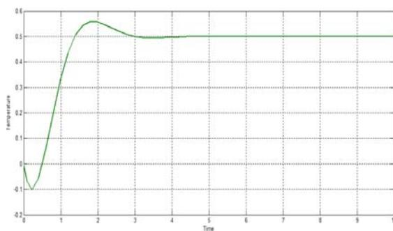
Figure 7. Set point tracking of CSTR process with IMC Based tuned PI controller
