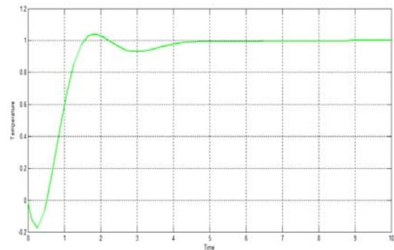
Figure 5. Set point tracking of CSTR process with Shen-Yu tuning PI controller
