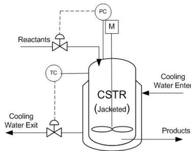
Figure 1. The Schematic of a CSTR
