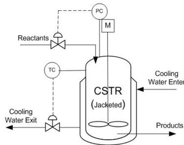
Figure 1. The Schematic of a CSTR
