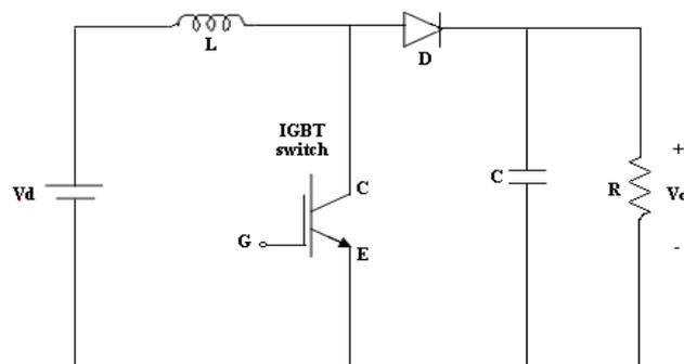
Figure 2. Circuit of the boost converter
