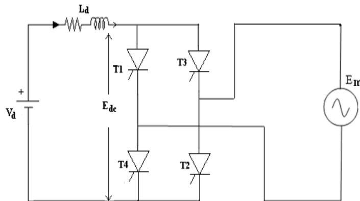
Figure 3. Circuit of the single-phase fully controlled bridge converter
