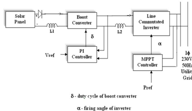
Figure 1. The block diagram schematic of the proposed scheme
