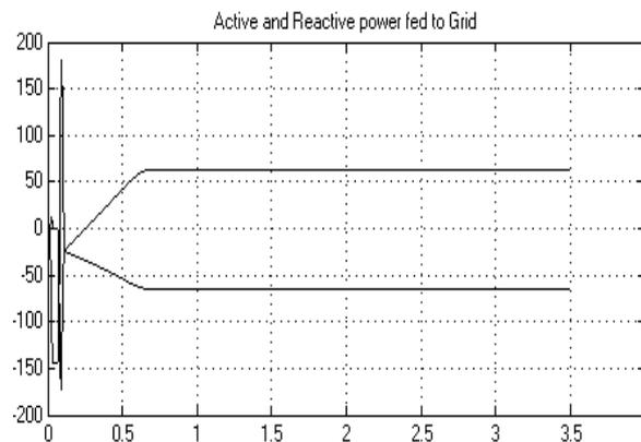
Figure 6. Active and Reactive power fed to the grid
