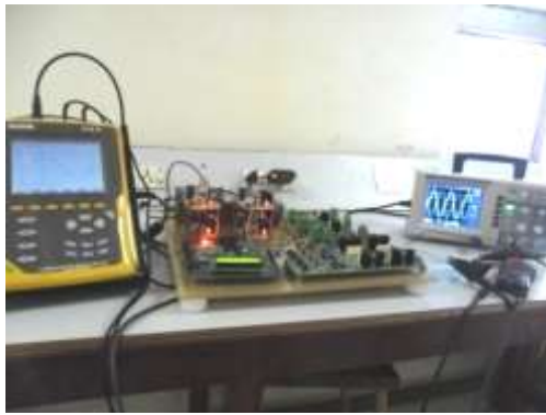
Figure 14. Hardware Setup of Symmetrical Multilevel Inverter
