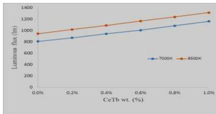
Figure 5. The lumen output at average CCTs 7000K and 8500 K with different CeTb concentration
