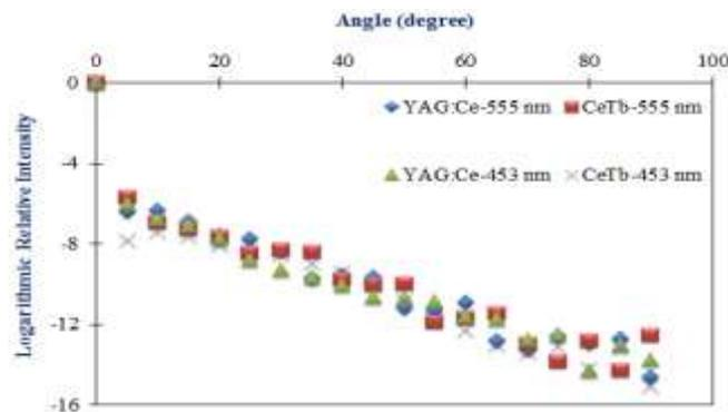
Figure 3. The light scattering distribution of CeTb and YAG:Ce particles in the phosphor layer of MCW-LEDs for 453 nm and 555 nm
