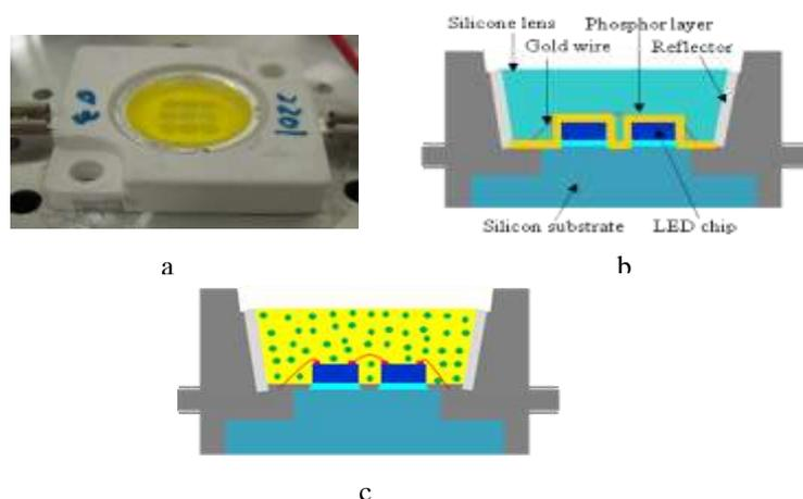
Figure 1. (a) The actual MCW-LED with in-cup phosphor layer, (b) Its schematic cross-sectional view, (c) The simulated in-cup phosphor packaging (CPP)
