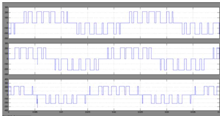
Figure 11. Inverter Output Voltages of Va, Vb, Vc
