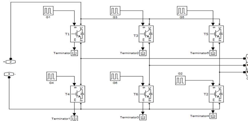
Figure 8. Subsystem of Voltage Source Inverter
