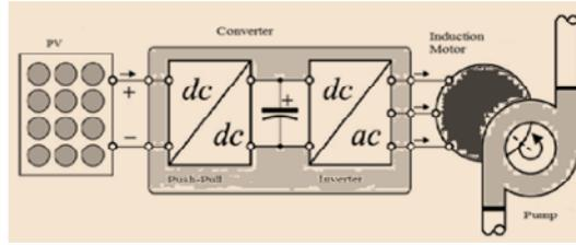
Figure 2. Photovoltaic pumping systems
