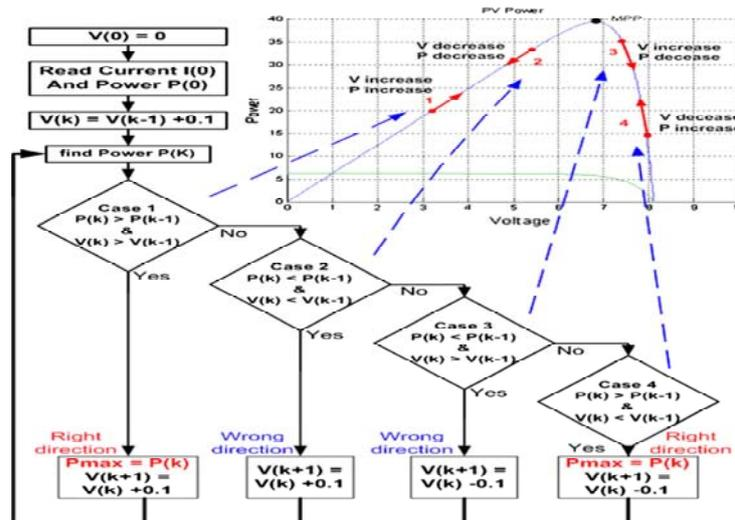
Figure 5. Perturb and observe MPPT technique
