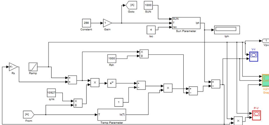
Figure 7. Subsystem of PV Cell
