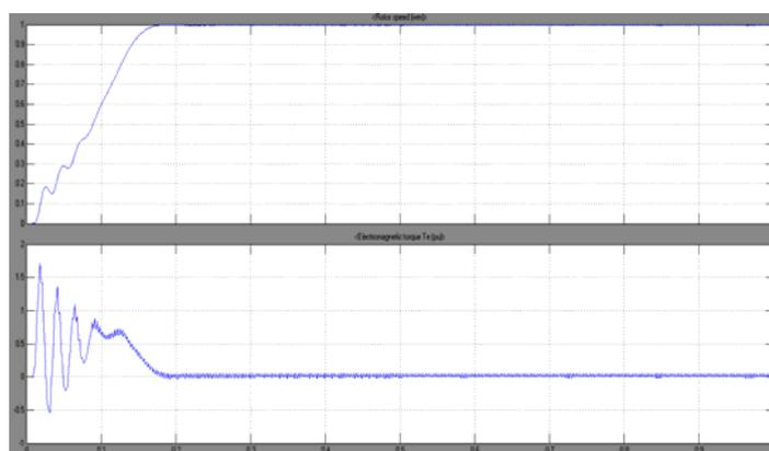
Figure 12. Speed and Torque characteristics Induction motor
