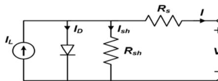
Figure 4. PV cell equivalent diagram
