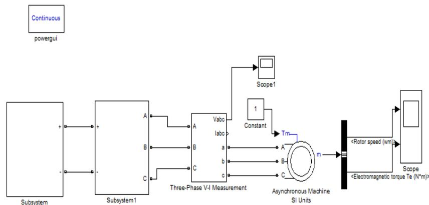
Figure 6. Complete system simulation Diagram of PV Cell Fed induction Motor
