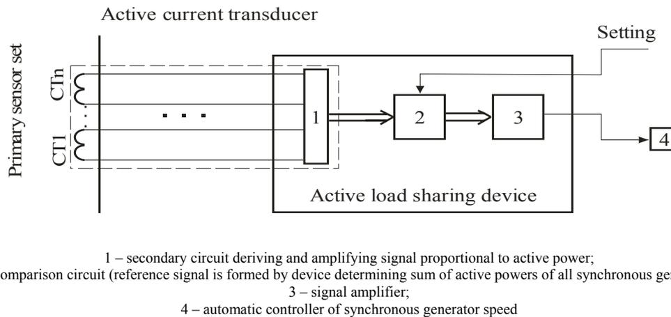
Figure 1. Typical functional diagram of synchronous generator active power controller
