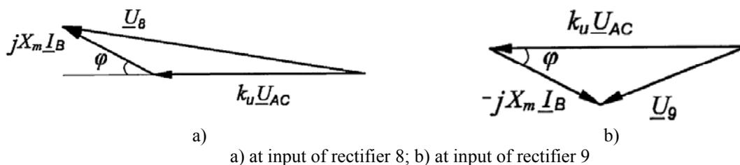
Figure 3. Phasor diagrams of currents and voltages
