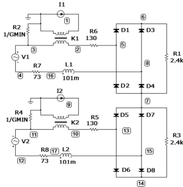
Figure 4. Simulation diagram of device for measurement of active current
