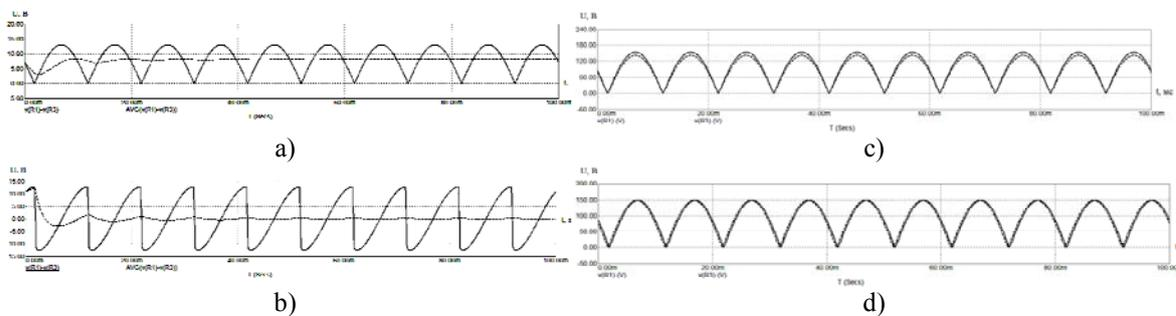
a, c – instantaneous value (solid line) and mean value (dotted line) of voltage on output of transducer at balanced resistive and inductive load ( $I = 50$  A); b, d – graphs of instantaneous voltages on resistors R1 (solid line) and R3 (dotted line) at balanced resistive and inductive load ( $I = 50$  A)
