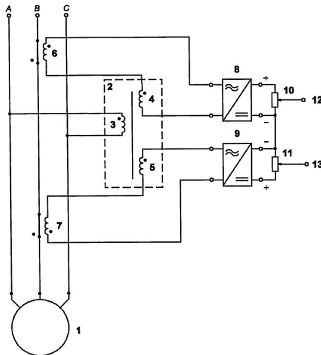
1 – synchronous generator; 2 – voltage transformer; 3 – primary winding of voltage transformer; 4, 5 – secondary windings of differentiating inductive current transducers; 6, 7 – differentiating inductive current transducers; 8, 9 – single-phase bridge rectifiers; 10, 11 – adjustable resistors; 12, 13 – output terminals of active current measurement device
